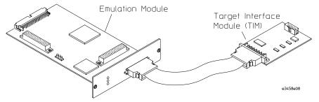
You can connect the emulation module to an analysis probe or you can connect it to a debug port on the target system through the provided target interface module (TIM).
