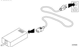
**2** Connect the 12V power cord to the back of the emulation probe.
